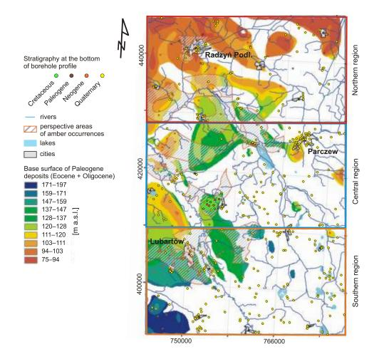
Fig. 2. Map showing the location of boreholes from which data have been used to create a vertical lithotype proportion diagram (VLPD) for the whole area, covering the sheets
