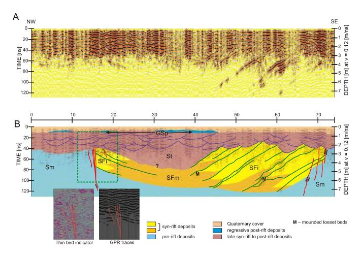
Fig. 12A. 2D GPR section parallel to the sand pit's outcrop wall trending NW–SE (see location in Fig. 4); B – interpretation of the GPR section in terms of sedimentary facies architecture, verified by observations from the outcrop wall; the inset images show the GPR signature of synsedimentary faults and related fractures
