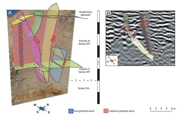
Fig. 9A. 3D model of the foreset of facies SFi with synsedimentary normal faults and fractures; based on GPR imagery combined with multiple-point statistics (numerical impala algorithm); B – GPR image of fault escarpment at the western graben margin
