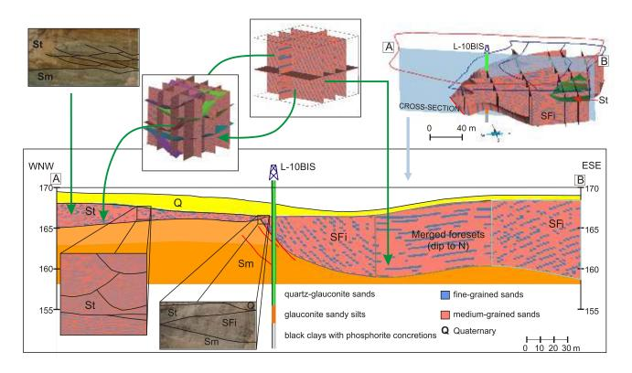
Fig. 11. Reconstruction of the spatial facies relationships and stratification architecture in the study area derived from surface-based modelling and multiple-point statistics
