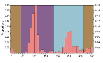
Fig. 7. Histogram of the dip azimuths of giant foreset stratification (facies SFi) derived from GPR data and outcrop measurements
