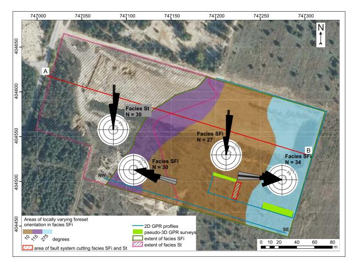
Fig. 6. Facies map of the detailed study area in Nowodwór-Piaski open-pit mine (see red frame in Fig. 1C), showing spatial changes in the direction of inclined stratification in facies SFi documented by measurements in the course of progressive mining
