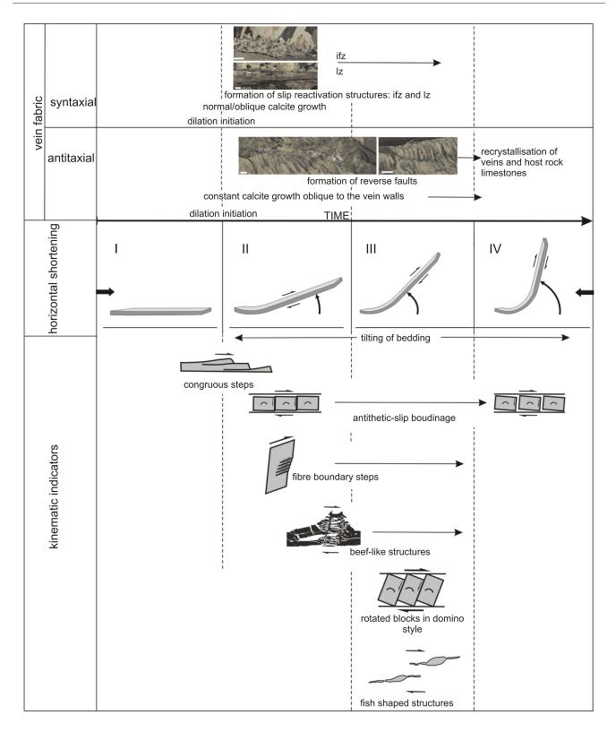
Fig. 11. Proposed model of bedding-parallel vein formation
