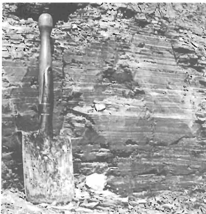
Fig. 3. Fragment of varved clay exposure in the brickyard (varved clays horizontally bedded); photo by E. Myślińska
