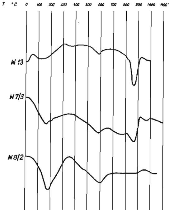
Fig. 2. Thermograms of selected samples (W13, W7/3, W8/2) of cohesive soils, grain size  $<0.25$  mm
