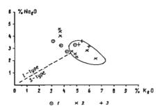
Fig. 4. K<sub>2</sub>O:Na<sub>2</sub>O diagram with marked field of projection points occurrence of Finnish rapakiwi granites (I. Haapala et al., 1987) along with division into fields of I-type and S-type granitoids
