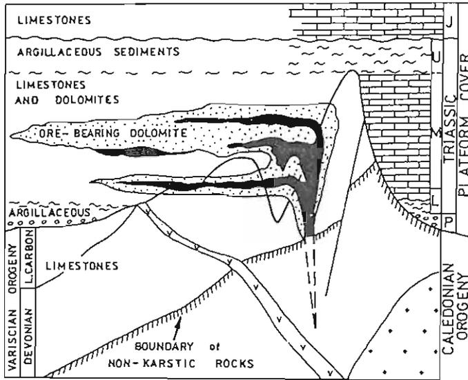
Fig. 2. Scheme of hydrothermal karst system related the structural units of the Silesian-Cracow Zn-Pb ore district (after M. Sass-Gustkiewicz, in press)
