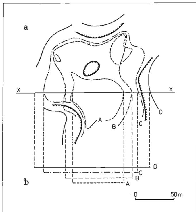
Fig. 1. Horizontal section through collapse breccia showing zonal distribution of various stages of mineralization, indicated from the oldest A, B, C and D respectively (a) and areas occupied by succeeding stages of mineralization along the cross-section line x — x (b); indented line indicates breccia boundary (modified after M.Sass-Gustkiewicz, 1975)
