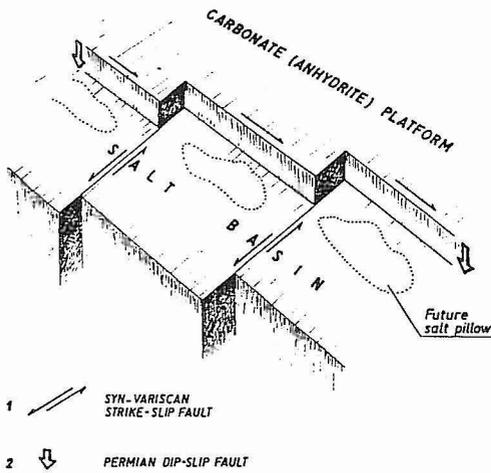
Fig. 7. Simplified sketch of the block arrangement in the Zechstein
