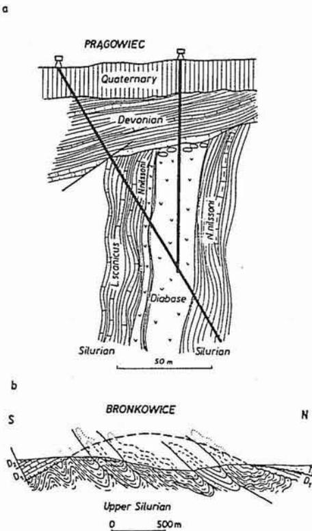
Fig. 3. a — Diabase sill within the Silurian and the sub-Devonian angular unconformity — Kielce Unit (after Z. Kowalczewski, R. Lisik, 1974, simplified); b — Sub-Devonian angular unconformity — Łysogóry Unit (J. Znosko after the data in J. Czarnocki, 1957 and E. Mariańczyk, 1973)
