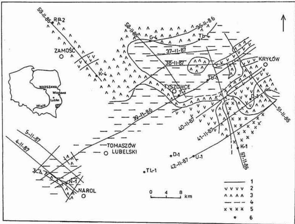
Fig. 1. Location of seismic profiles against the background of a sketch showing distribution of velocity of wave propagation in the formation below the bottom of the Low Velocity Zone (LVZ)
