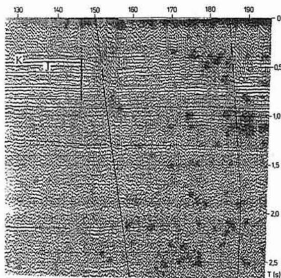
Fig. 18. Zones of tectonic disturbance on the profile 58-II-86, occurring on segments of diversified relief of land surface
