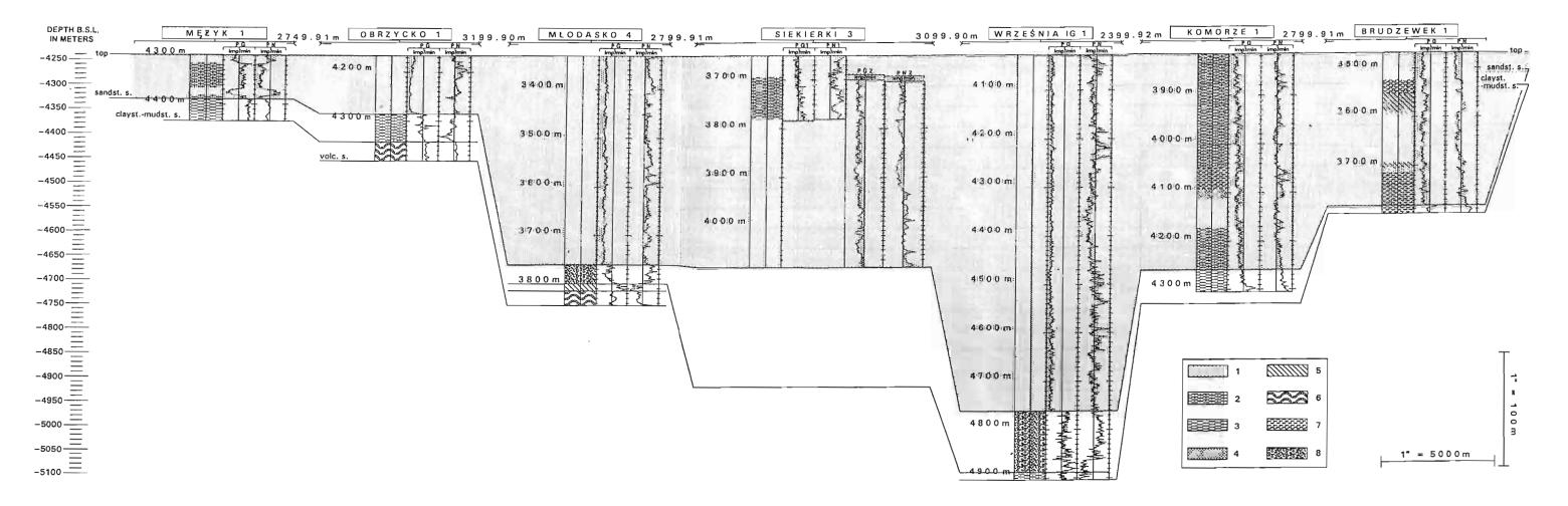
Fig. 7. Correlation of lithological series identified in wells along profile II-II (apart from Sobieseki 2 and Gomunice 6); top of Rotliegend means the reference level; lithological rock profile constructed basing on geophysical interpretation
