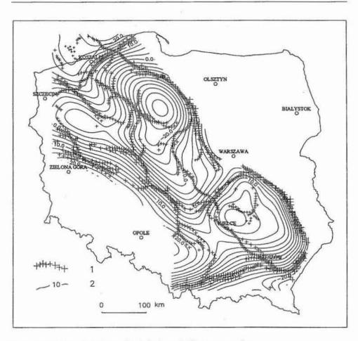
Fig. 2. Axes of horizontal gradient againts the background of Bouguer anomalies
