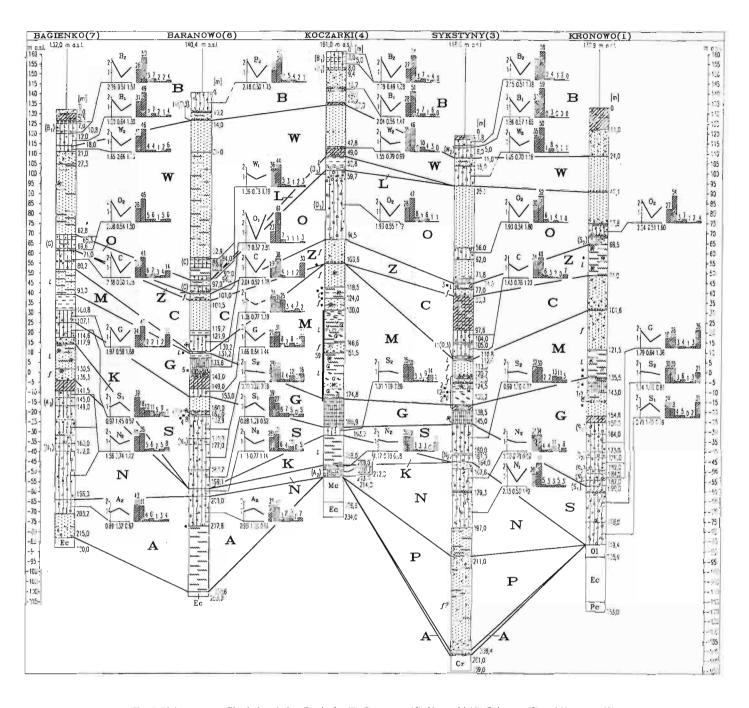
Fig. 4. Pleistocene profiles in boreholes: Bagienko (7), Baranowo (6), Koczarki (4), Sykstyny (3) and Kronowo (1) Explanations as in Fig. 2
