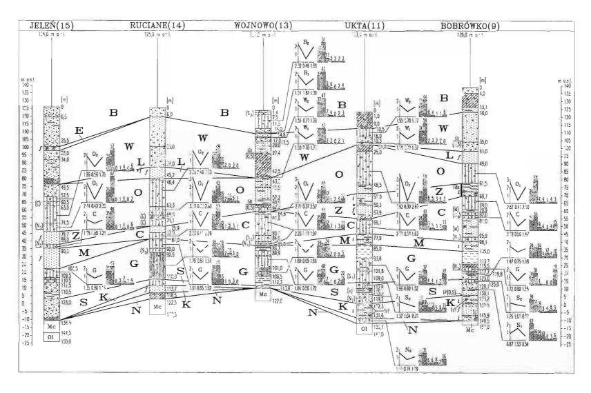
Fig. 3. Pleistocene profiles in boreholes: Jeleń (15), Ruciane (14), Wojnowo (13), Ukta (11) and Bobrówko (9) Explanations as in Fig. 2
