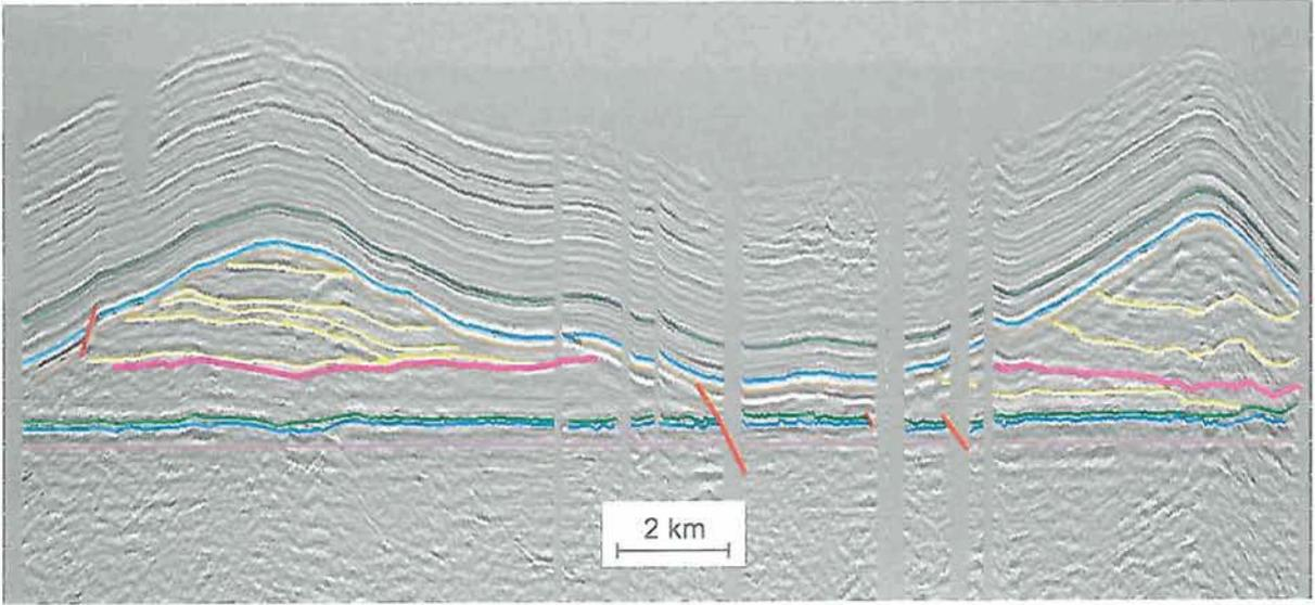
Fig. 5. Interpreted time seismic line 24-5-80K flattened on seismic horizon related to top of the Lower Devonian
