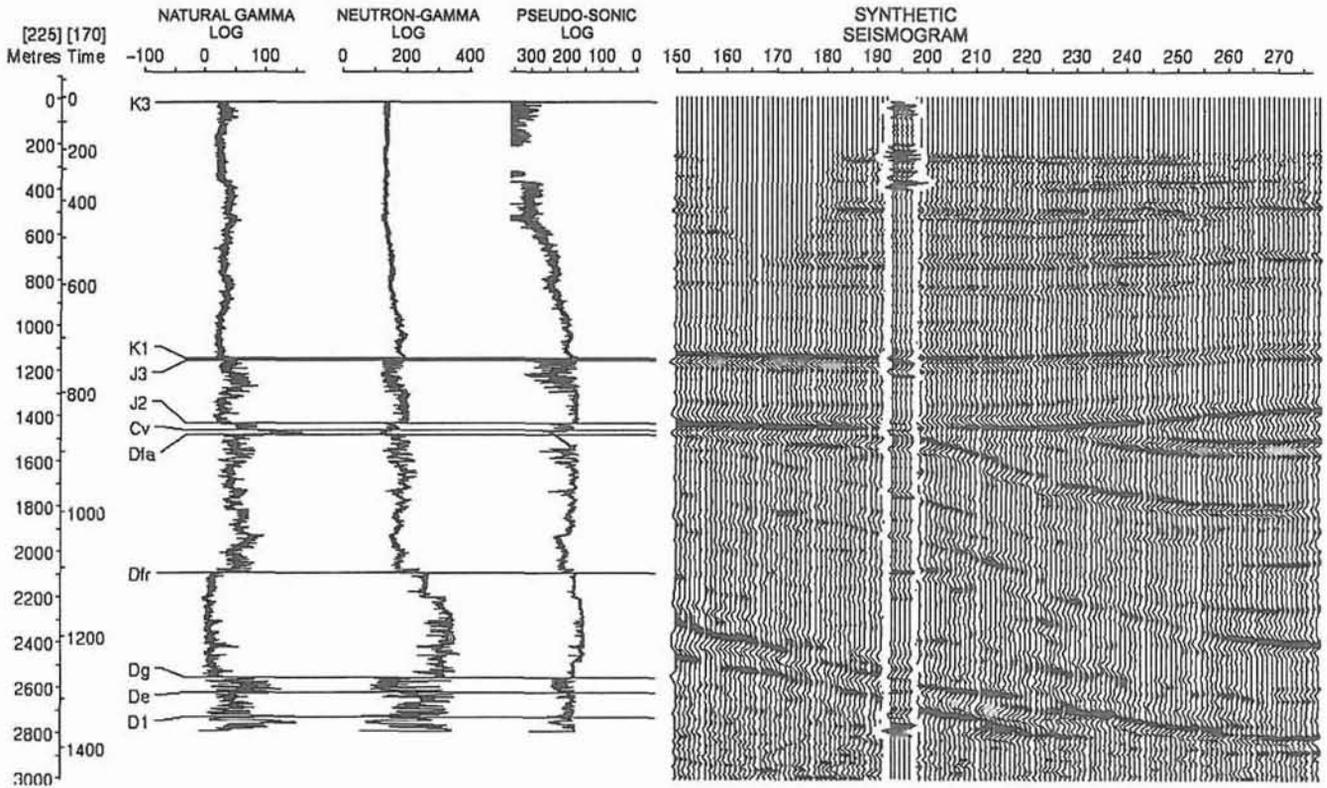
Fig. 3. Well Zakrzew IG 1 — natural gamma-ray log, sonic log, synthetic seismogram and its correlation with part of seismic line 24-5-80K
