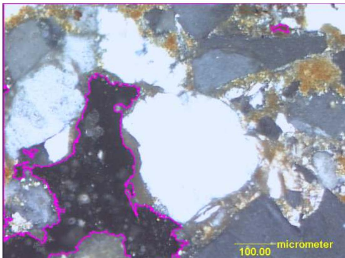
Fig. 1. Contoured pore area in sample 2 (magnification x 100)
