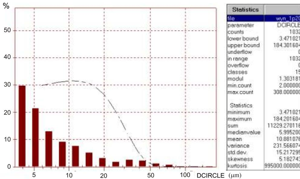
Fig. 2. Histogram of diameters of equivalent area circles for the sample 1
