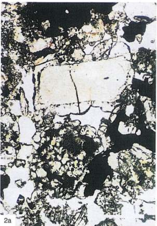
1a. Different types of chondrules; in the center a sibling porphyritic chondrule with a large automorphic olivine crystal; polished thin section B-10, area 11, chondrules 28 and 29; scale bar 0.25 mm. 1b. As above, crossed nicols. 2a. An individual automorphic olivine with an epitaxial rim; polished thin section B-10, area 3, chondrule 15, and olivine; scale bar 0.25 mm. 2b. As above, crossed nicols
