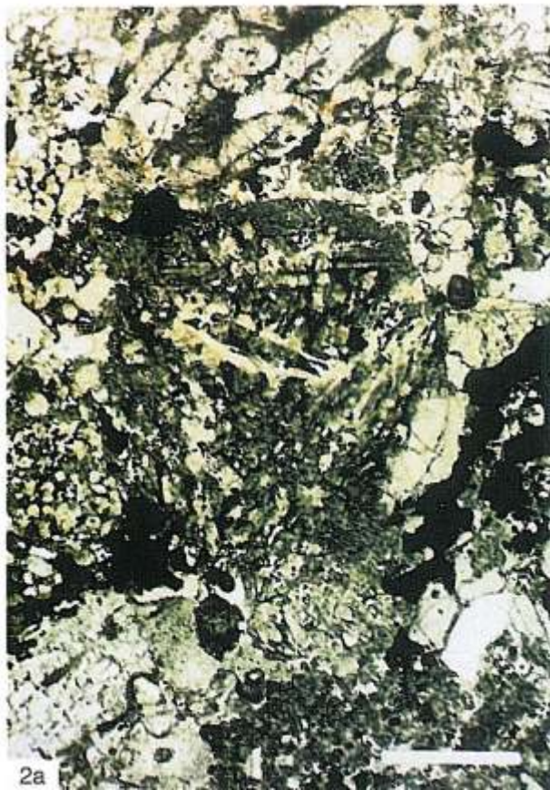
1a. A sectorial porphyritic chondrule with a twinned pyroxene; polished thin section B-10, area 26, chondrule 1; scale bar 0.5 mm. 1b. As above, crossed nicols. 2a. A poikilitic pyroxene-olivine chondrule among fragments of different chondrule types; polished thin section B-10, area 17, chondrules: 1, 11 and 28; scale bar 0.5 mm. 2b. As above, crossed nicols
