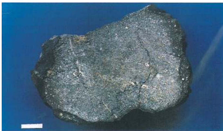
Fig. 2. Baszkówka meteorite — the external surface of plate b from Fig. 1A; at left — a large metal-troilite particle, and a long chain of metal grains; at right, next to a fracture — four small metal-troilite particle; scale bar 20 mm
