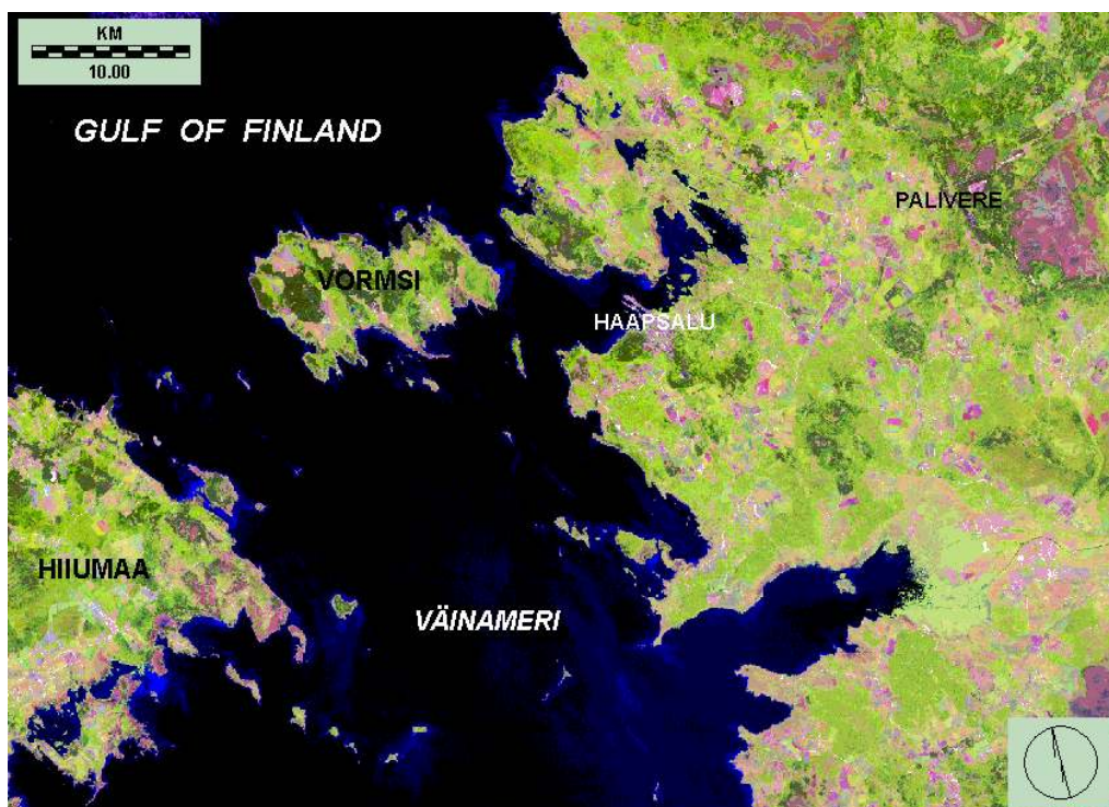
Fig. 2. Landsat TM composite made of bands 3, 4 and 5, colour coded as blue, green and red, 28 July 1986; dark blue and black — water bodies, dark green — spruce forest, reddish-green — pine forest, yellowish-green — deciduous forest, pink and purple — agricultural fields, white — cultural structures (roads and villages)
