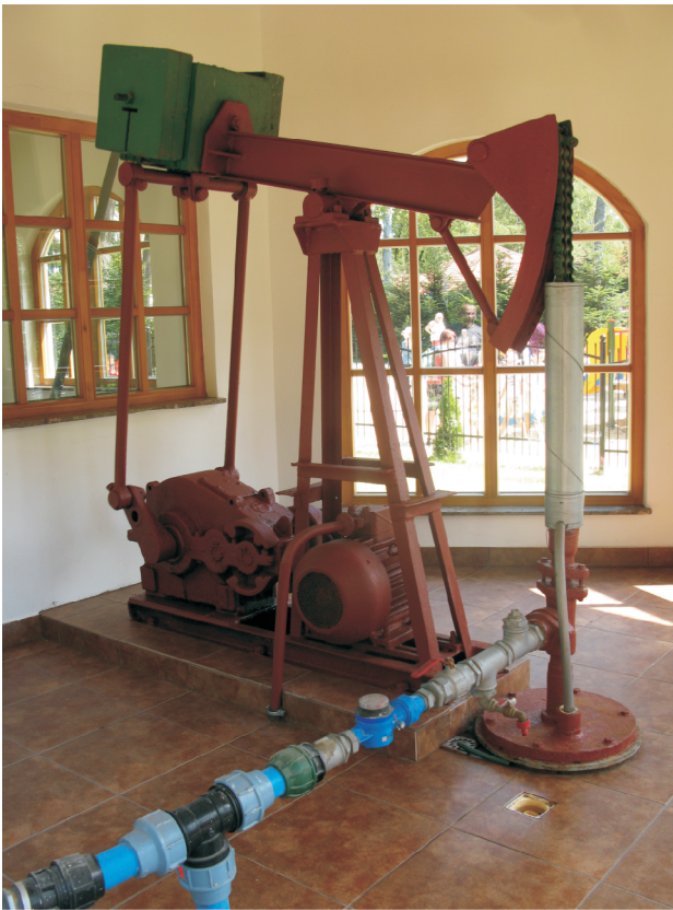
Fig. 2. Helena borehole with a rod-type “Konik” pump (photo by L. Rajchel)
