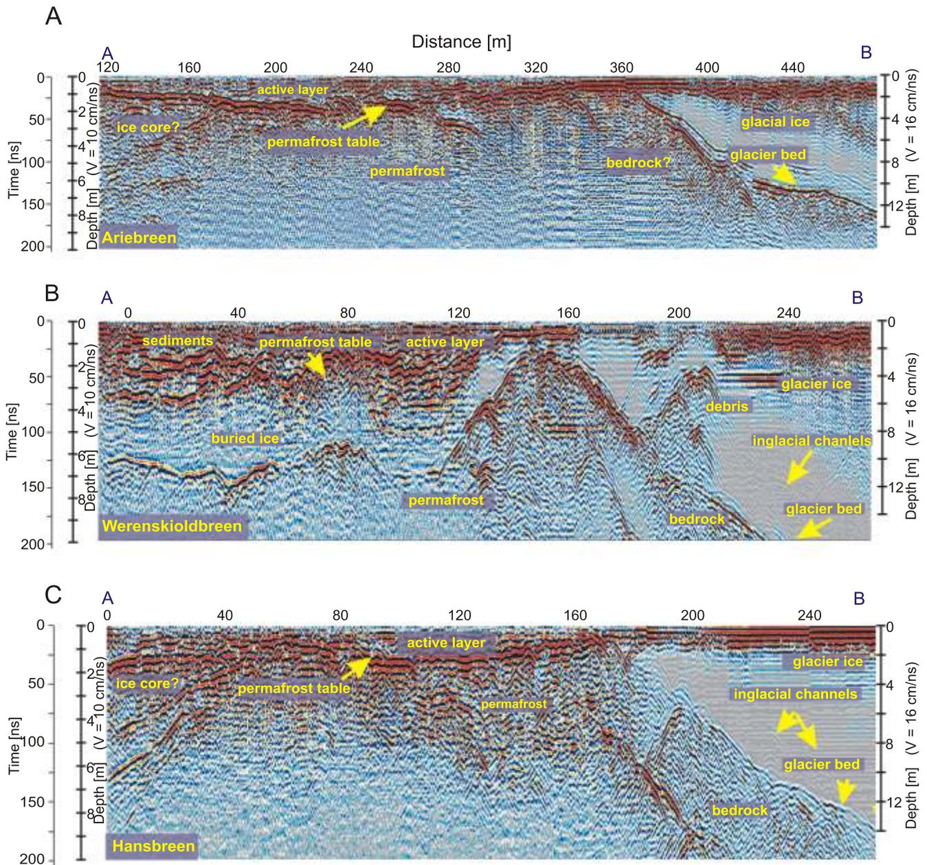
**Fig. 6. Results of the GPR profiling performed on Ariebreen (A), Werenskioldbreen (B) and Hansbreen (C), and its forefields, Hornsund area, Spitsbergen**
