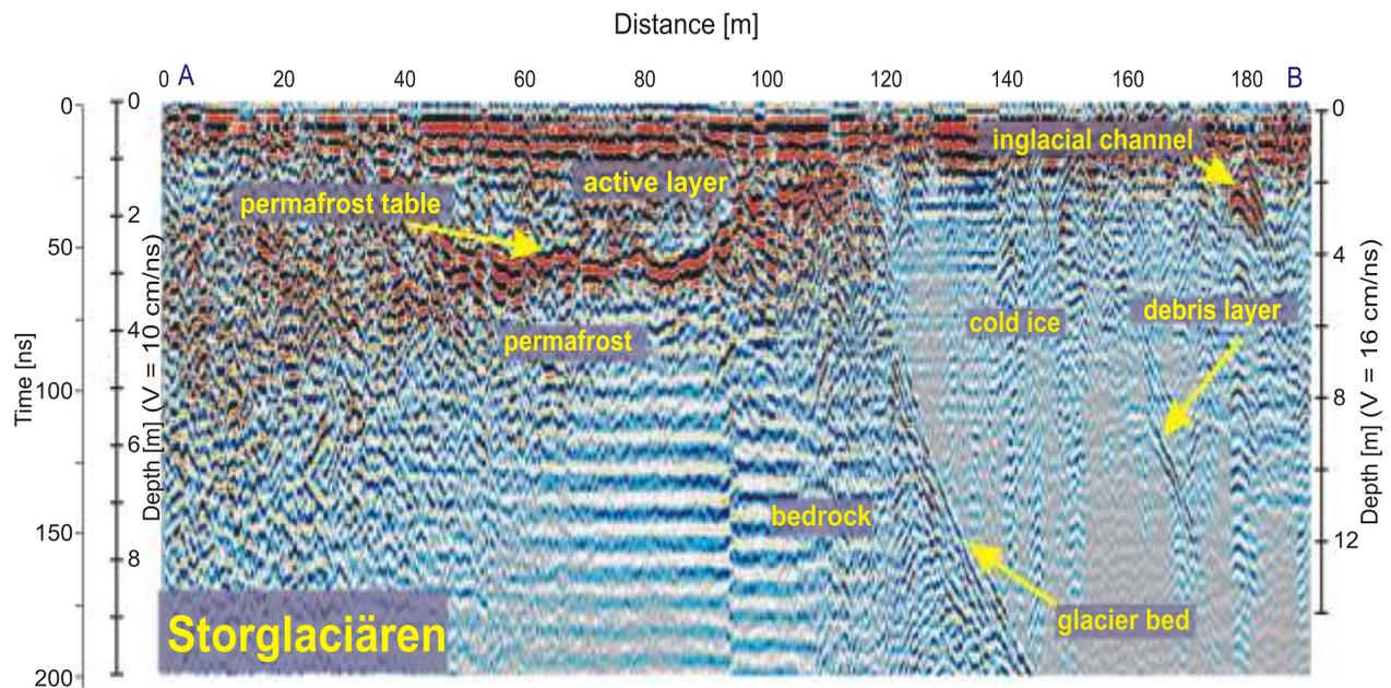
Fig. 5. Result of the GPR profiling performed on Storglaciären and its forefield, Kebnekaise Massif, Northern Sweden
