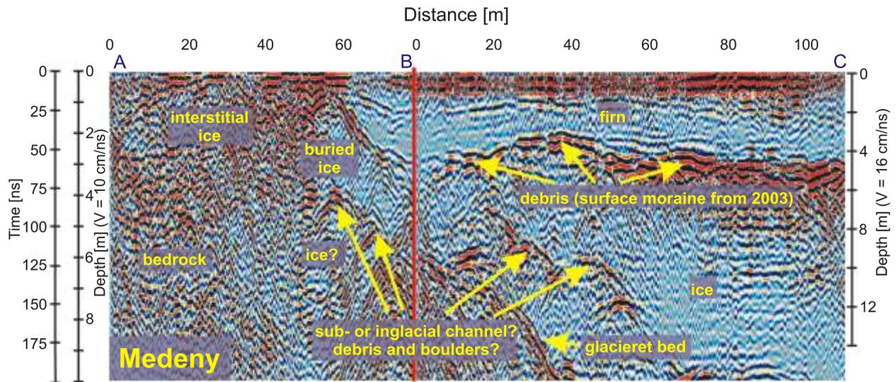
Fig. 4. Result of the GPR profiling performed on the Medeny glacieret and its forefield, Medena kotlina, Tatra Mts., Slovakia
