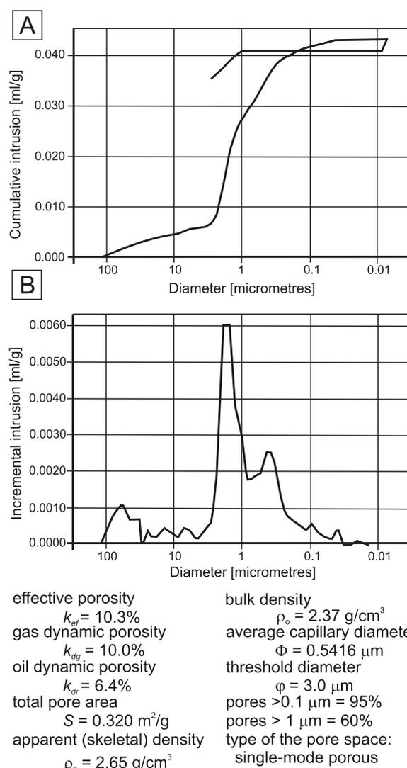
Fig. 2. Mercury porosimetry results
