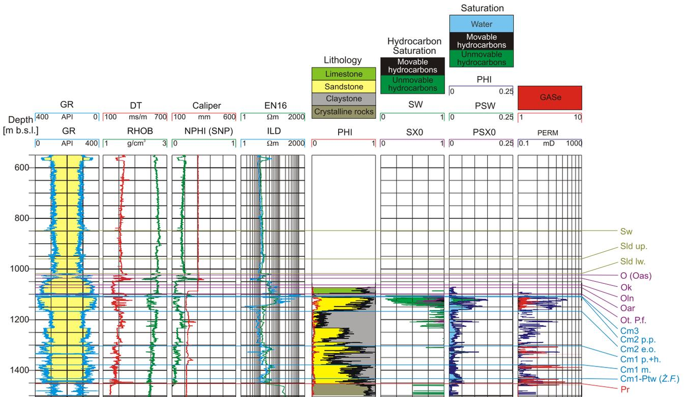
Fig. 10. Logs and results of the comprehensive interpretation of the B4-1/81 borehole (Profile III)
