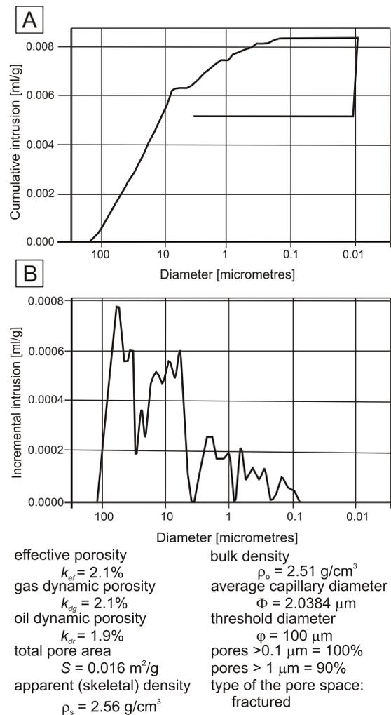
Fig. 6. Mercury porosimetry results
