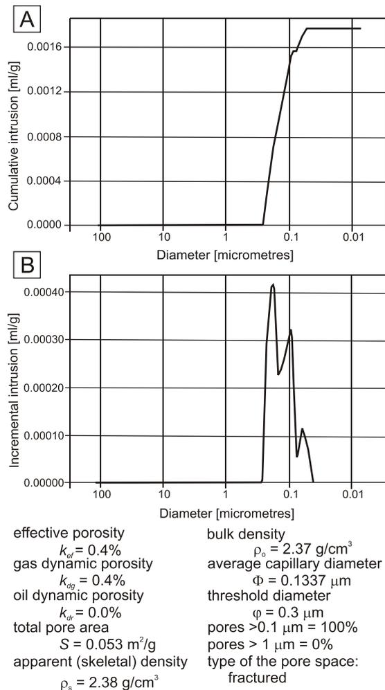
Fig. 7. Mercury porosimetry results
