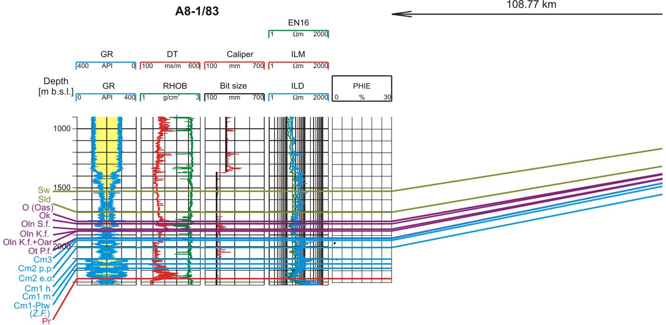
Fig. 9. Logs in the A8-1/83, B6-3/02 and B6-1/82
