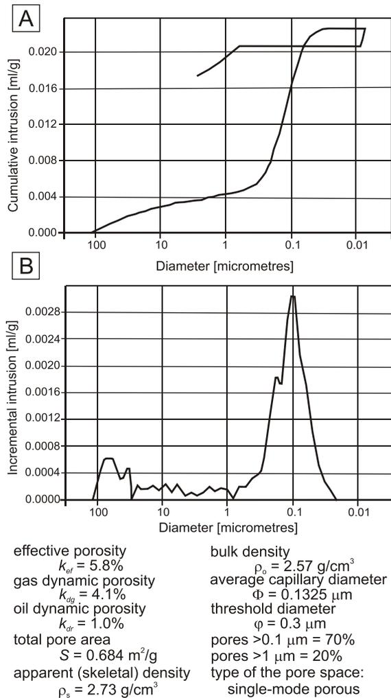
**Fig. 3. Mercury porosimetry results**
