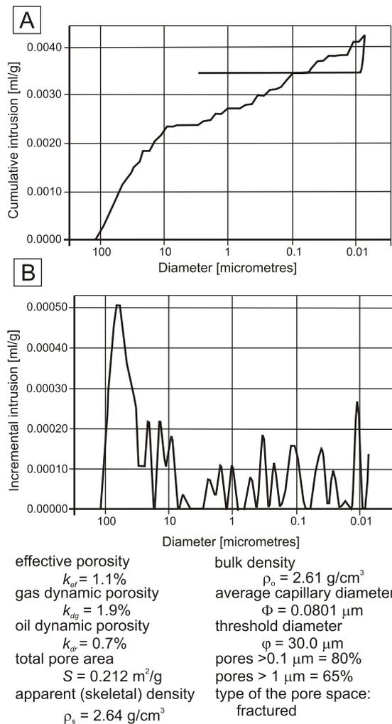
Fig. 5. Mercury porosimetry results
