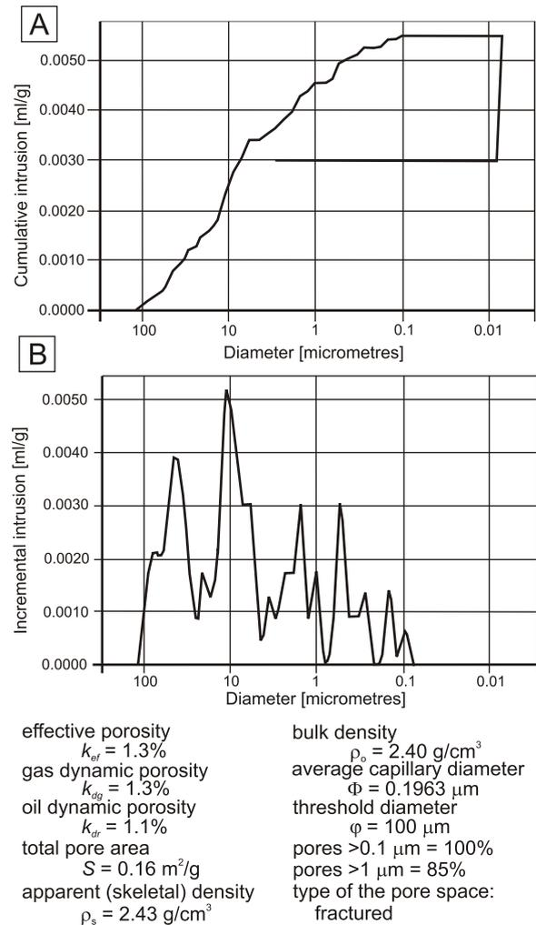
**Fig. 4. Mercury porosimetry results**
