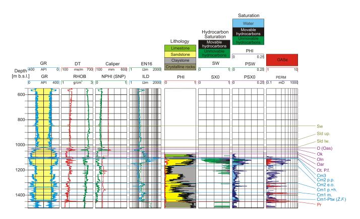
Fig. 10. Logs and results of the comprehensive interpretation of the B4-1/81 borehole (Profile III)
