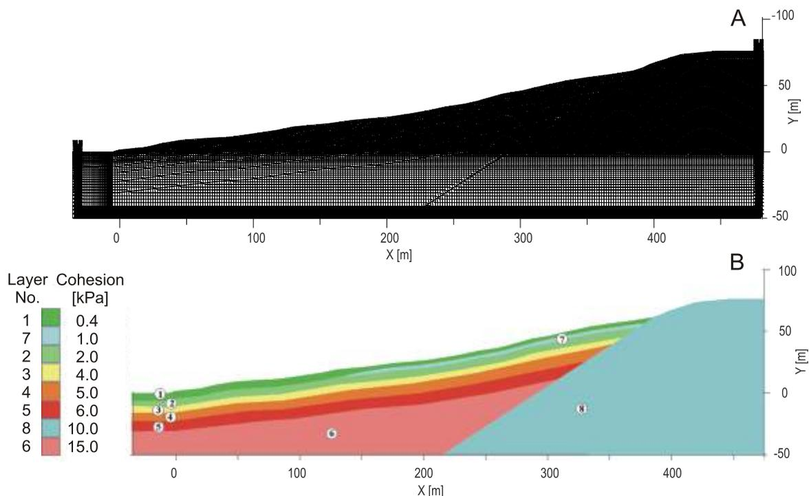
Fig. 12. Numerical model of the Kawiory landslide system
