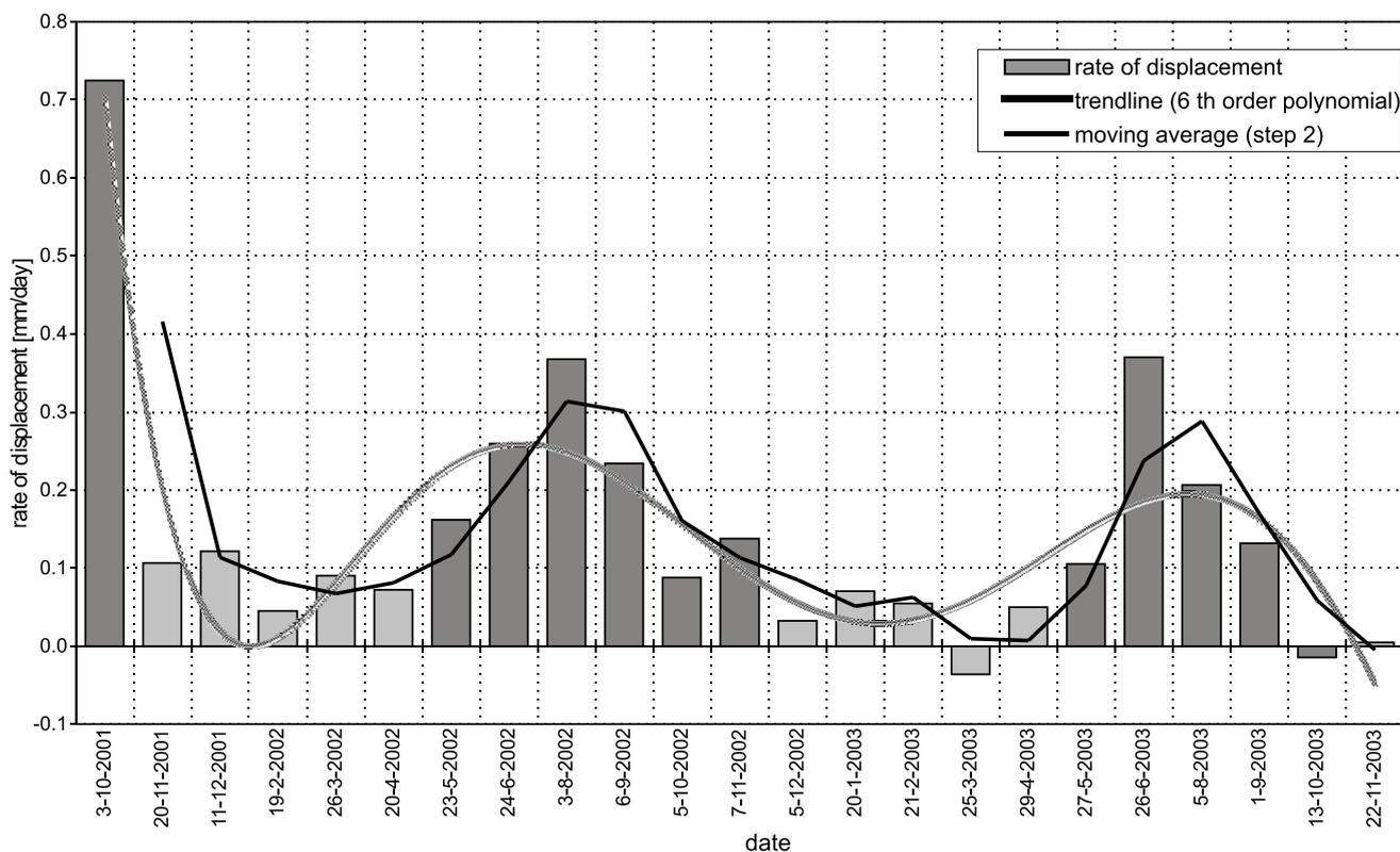
Fig. 9. Displacement rate in borehole K3
