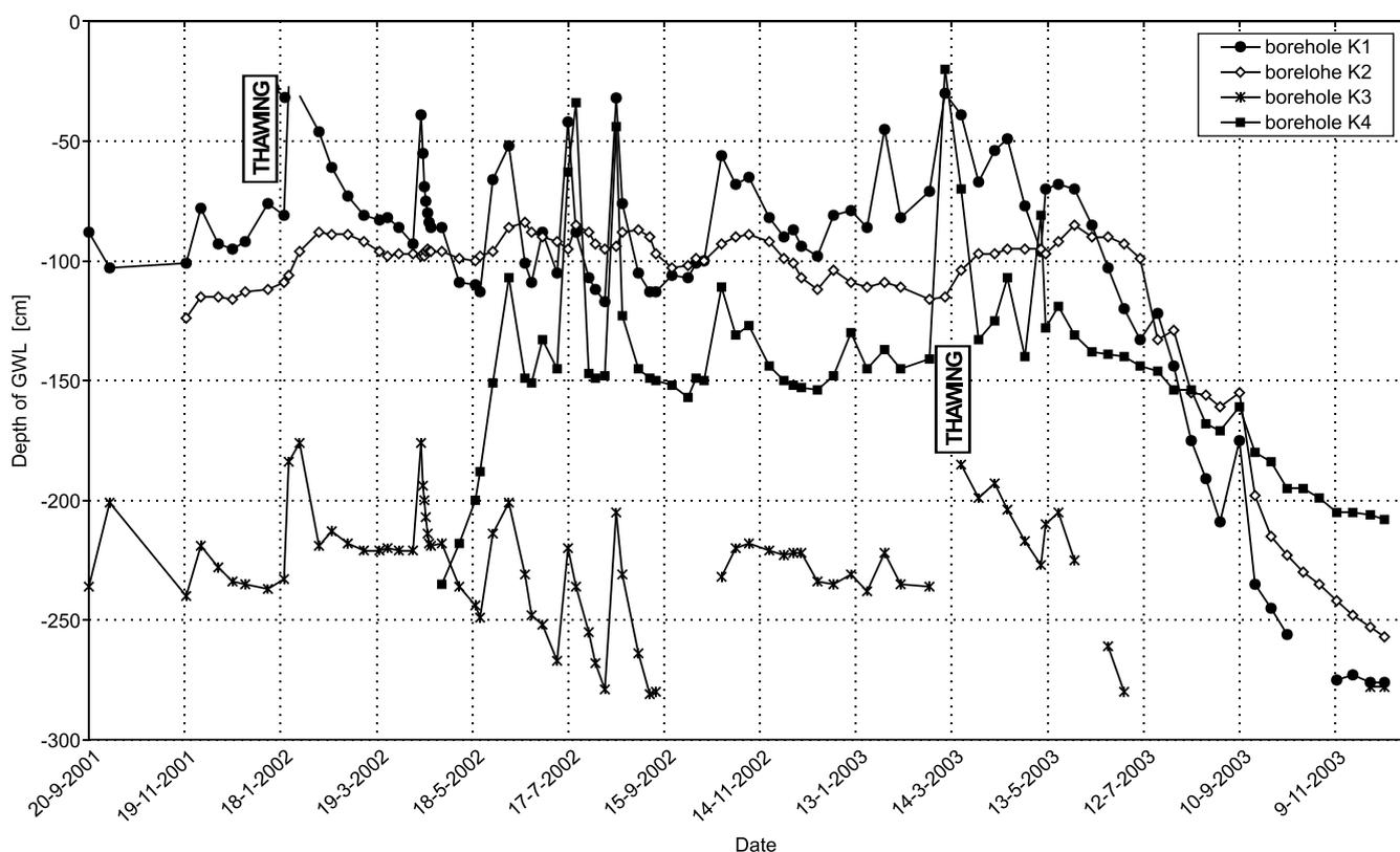
Fig. 7. Groundwater level measured in piezometers
