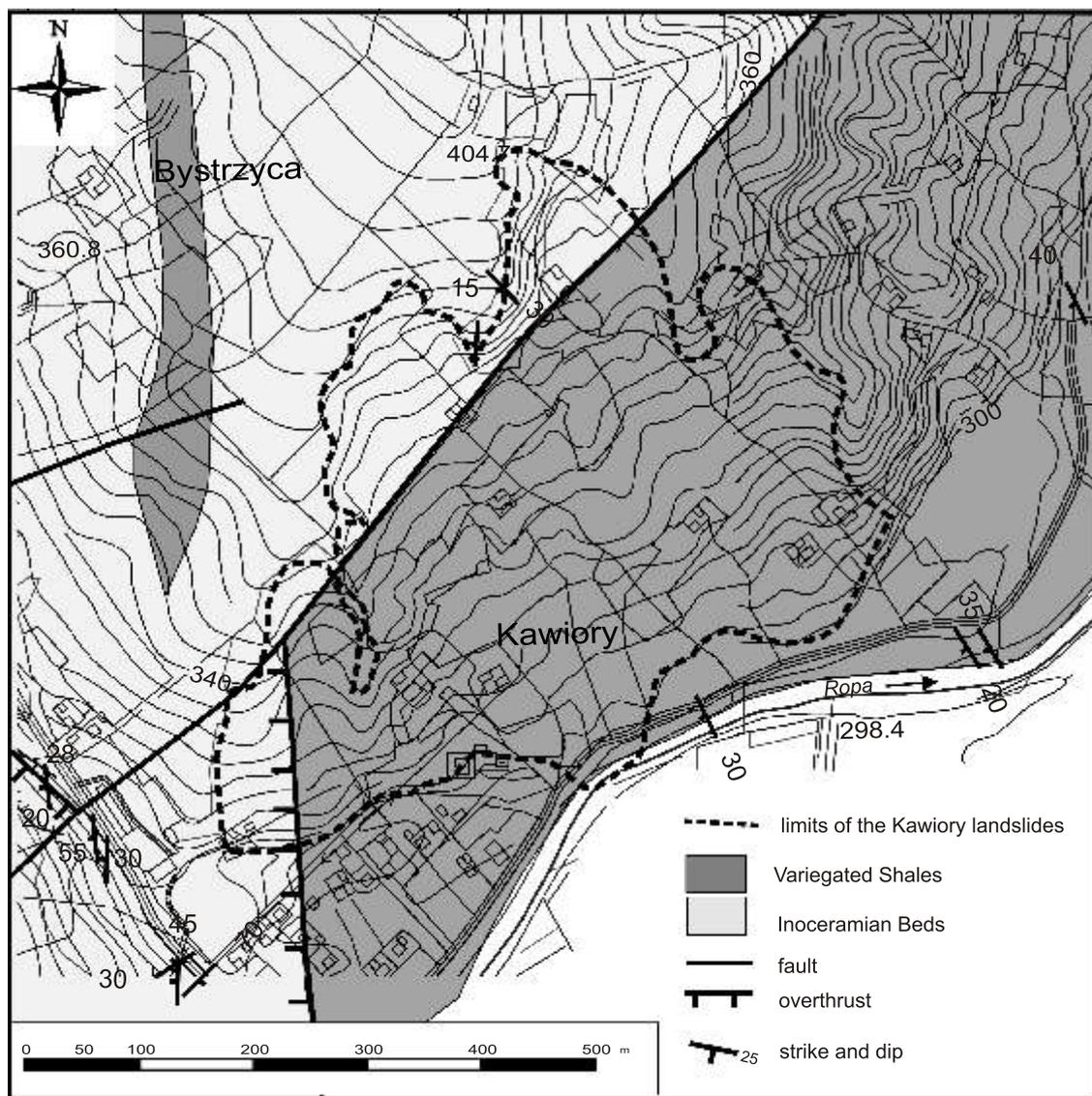
Fig. 3. Geological sketch and Kawiory landslide system (after Wójcik, 2002)
