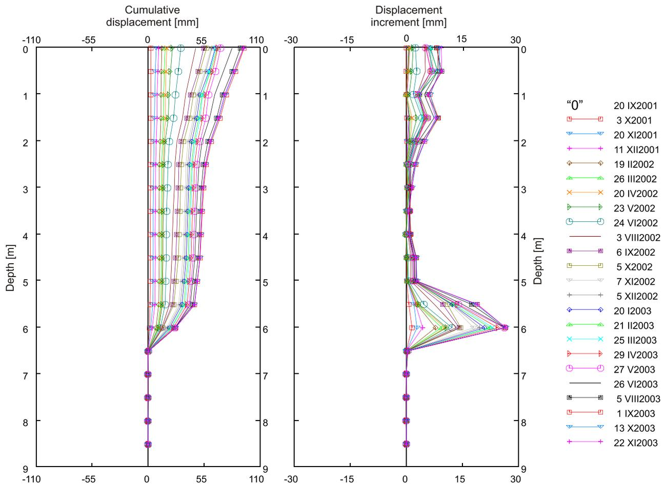
Fig. 8. Cumulative and incremental displacement measured by inclinometer in borehole K3
