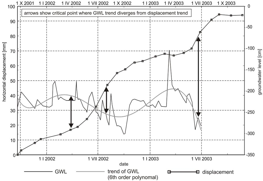
Fig. 10. Groundwater level and horizontal displacement in borehole K3
