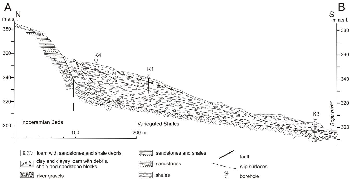
Fig. 5. Geological cross-section of Kawiory landslide
