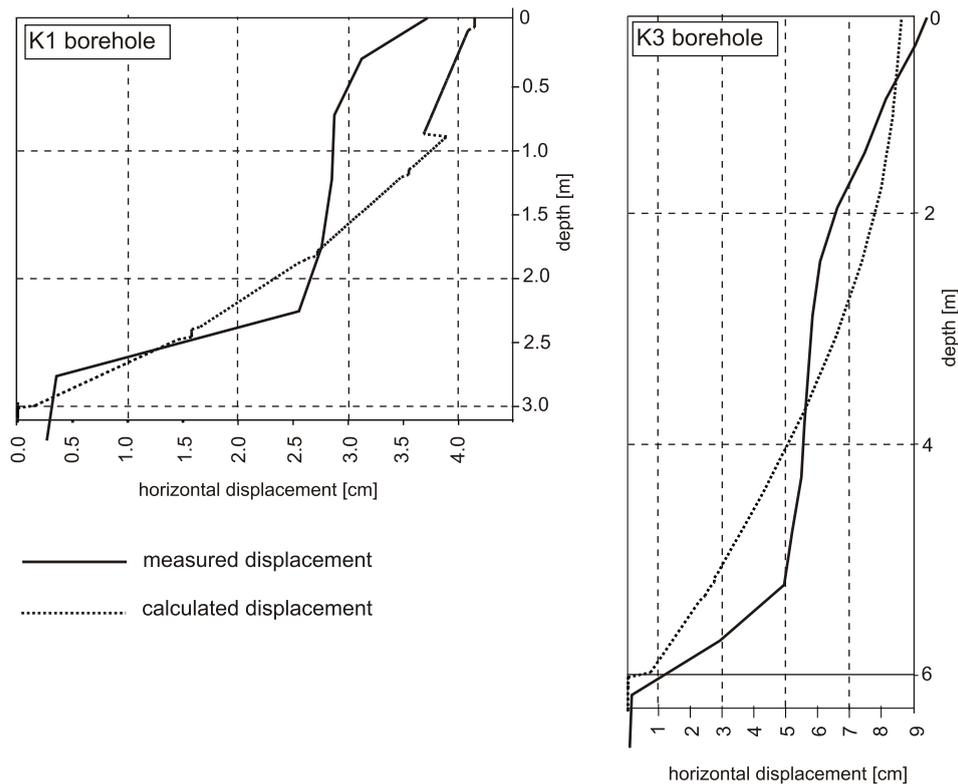
Fig. 14. Comparison of measured and calculated horizontal displacement in boreholes K1 and K3
