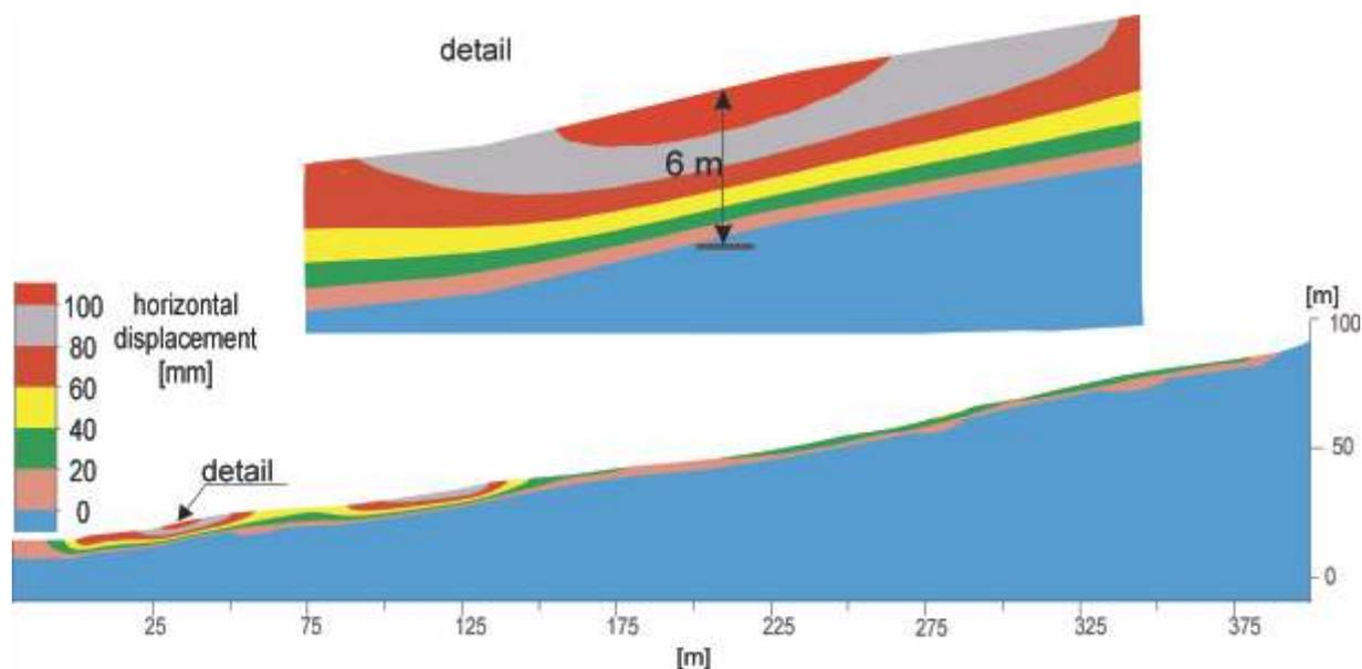
Fig. 13. Field of horizontal displacement after 2 years creep
