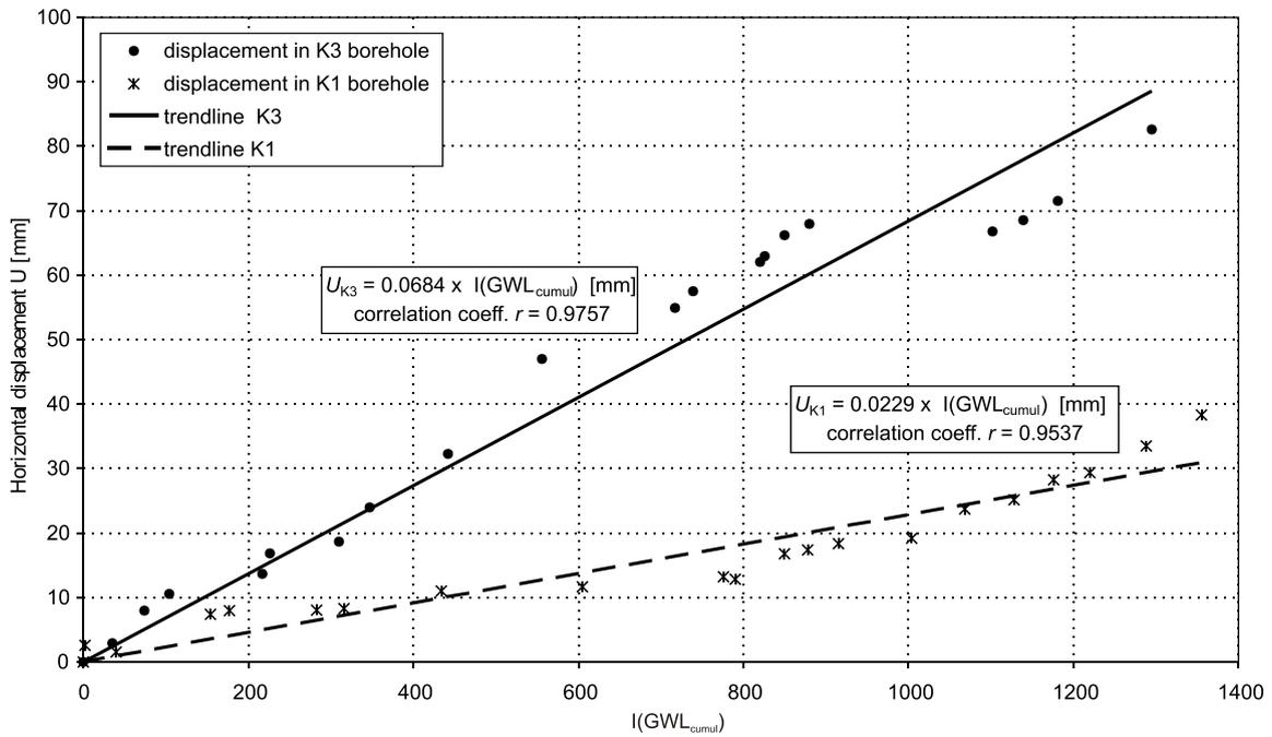
Fig. 11. Cumulative intensity of groundwater fluctuations versus horizontal displacement of K1 and K3 borehole, with regression formula and correlation coefficients
