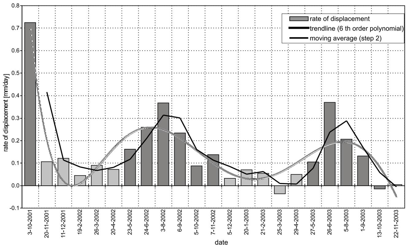
Fig. 9. Displacement rate in borehole K3
