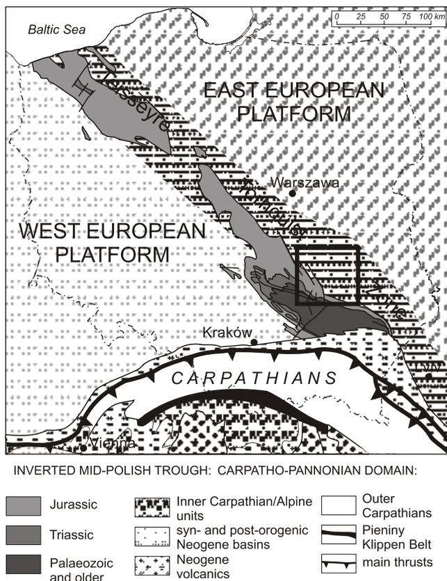
**Fig. 1.** Location of the study area (black rectangle) on a schematic map showing main tectonic units of Poland: NW–SE — trending inverted Mid-Polish Trough delineated by subcrops of the Jurassic and older rock, the Carpathians and the Carpathian Foredeep Basin
