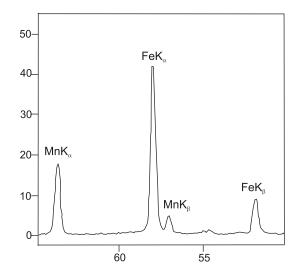
Fig. 6. Part of X-ray spectrum with Fe and Mn peaks, loess concretion from the Obrowiec section, sample 5
