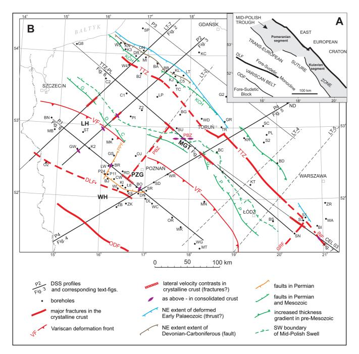
Fig. 1. A — geological sketch showing main tectonic features of the study area in NW Poland, B — location of studied deep seismic sounding profiles and analysed boreholes against tectonic features
