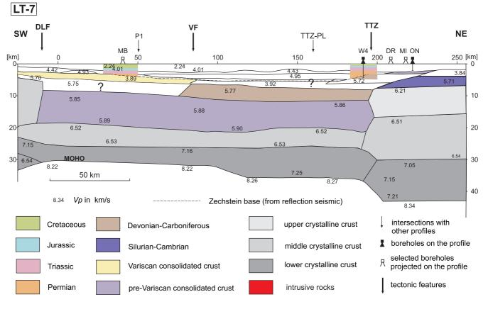
Fig. 2. Geological interpretation of the LT-7 deep seismic sounding profile
