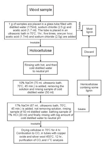
Fig. 4. The  $\alpha$ -cellulose extraction procedure used in Gliwice Radiocarbon Laboratory
