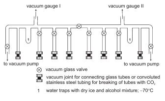
Fig. 7. The vacuum line for  $CO_2$  purification and preparation of samples for  $\delta^{13}C$  measurements in Gliwice Radiocarbon Laboratory
