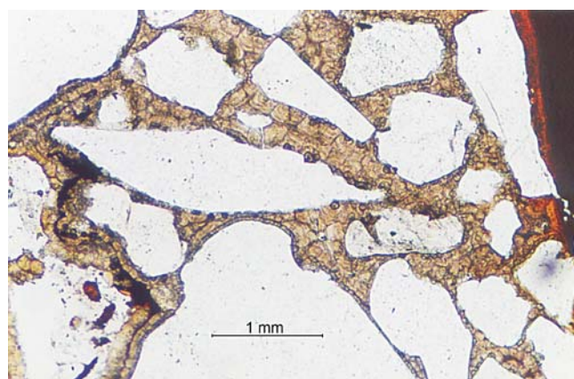
Fig. 4. Siderite with a lamellar and radial structure, binding clastic material, plane polarized light
