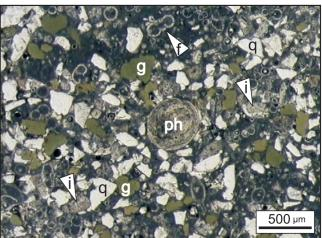
Fig. 12. Foraminiferal-inoceramid packstone with admixture of quartz and glauconite, microfacies of sandy-glauconitic limestone, upper lower Coniacian; ph—phosphate pellet; other explanations as on Figures 6 and 7
