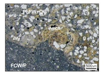
Fig. 7. Microfacies of the hardground zone. Phosphatized layer (phl) with micro-columnar phosphatic stromatolite (mcs) overlying the foraminiferal-calcisphere wackestone/packstone (FCW/P); PhFW + QG — phosphatized foraminiferal microfacies with admixture of quartz and glauconite; q — quartz, g — glauconite
