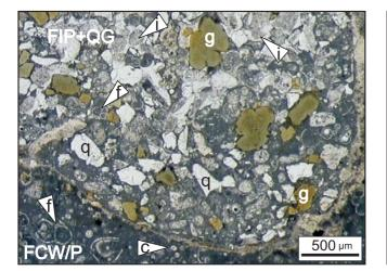
Fig. 11. Foraminiferal-inoceramid packstone with admixture of quartz and glauconite, upper lower Coniacian, infilling borings in the foraminiferal-calcisphere wackstone/packstone, upper Turonian; other explanations as on Figures 6–8
