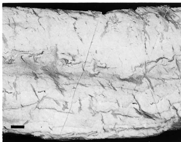
Fig. 9. Layered bed consisting of plastically deformed, normally graded, burrowed hard marlstone (light) grading into shale (thin, dark grey bedding-parallel laminae); lower part of Wiar section
