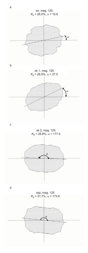
Fig. 3. Rose diagram of pore orientations
