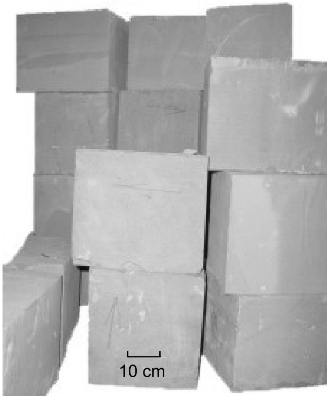
Fig. 3. Cubic blocks of Krosno Sandstones from Mucharz
