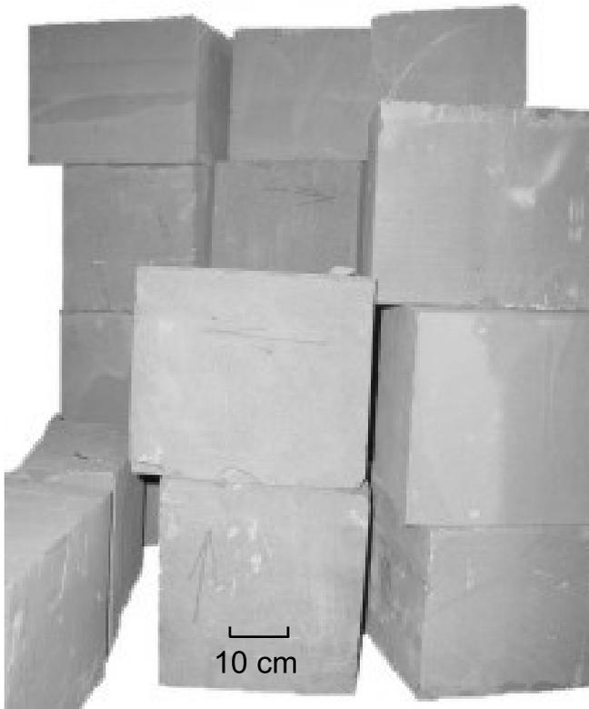
Fig. 3. Cubic blocks of Krosno Sandstones from Mucharz
