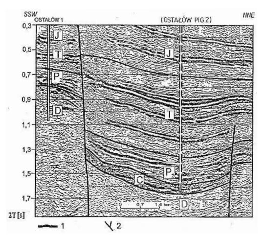
Fig. 5. Interpretation of reflection coefficient sections along a fragment of seismic profile 18-II/III-91, after Dziewi ska et al. (2000) (with the author's supplements)
