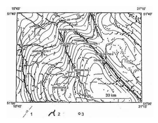
Fig. 2. Regional anomalies of the gravity field with density contacts (averaging radius r = 5 km, interval = 1 km), after Dziewi ska *et al.* (2000) 1 — isolines in  $10^{-5}$  m/s<sup>2</sup> (mGal); 2 — maxima of the modulus of horizontal gradient; 3 — selected boreholes
