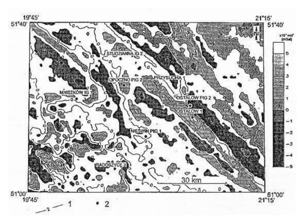
Fig. 3. Residual anomalies of the gravity field (averaging radius r = 5 km, interval = 1 km), after Dziewi ska *et al.* (2000) 1 — isolines in  $10^{-5}$  m/s<sup>2</sup> (mGal); 2 — selected boreholes
