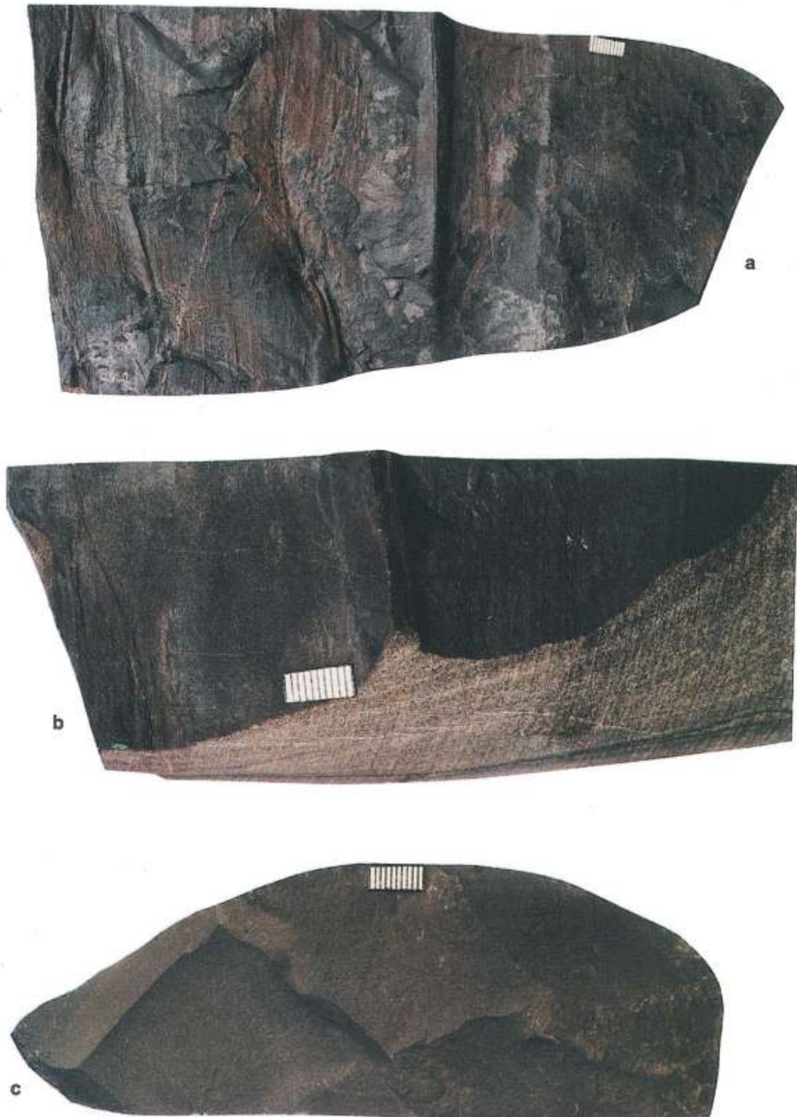
Fig. 8. a — facies 3; sole surface of thin fine-grained sandstone bed from sand/mud heterolith; mixed assemblage of current marks is visible: indistinct flute marks and tool marks, indicating turbulent flow depositing the sandstone bed; Ostałów PIG 2; depth 2518.5 m. b — facies 3; sole surface of sandstone bed from sand/mud heterolith; distinct tool mark is visible; overlying sandstone bed is visible at the bottom, owing to the cylindrical shape of the drillcore fragment; the bed shows small-scale cross lamination, resembling flaser bedding; Ostałów PIG 2; depth 2517.5 m. c — facies 4; dark clayey shale; Ostałów PIG 2; depth 2525.0 m
