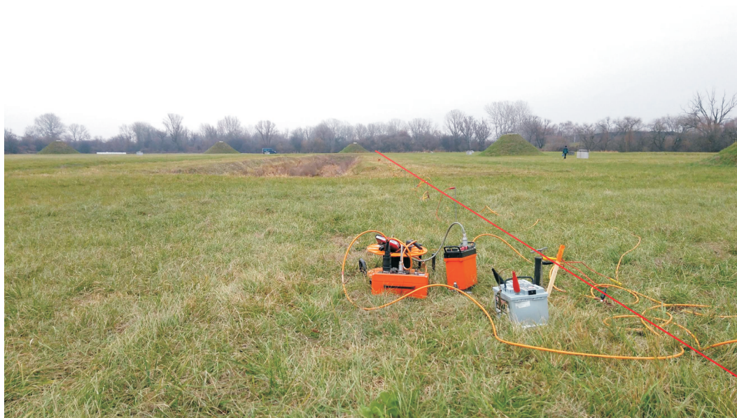
Fig. 2. LUND electrical imaging system with a Terrameter SAS 1000/4000 (ABEM Malå) used for the ERT measurements
