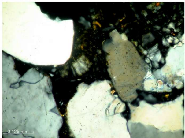
Fig. 7. Microscope images of samples LEG025, LEG028 and LEG033 in plane-polarized (left) and crossed-polarized light (right), illustrating detailed views of cements.
