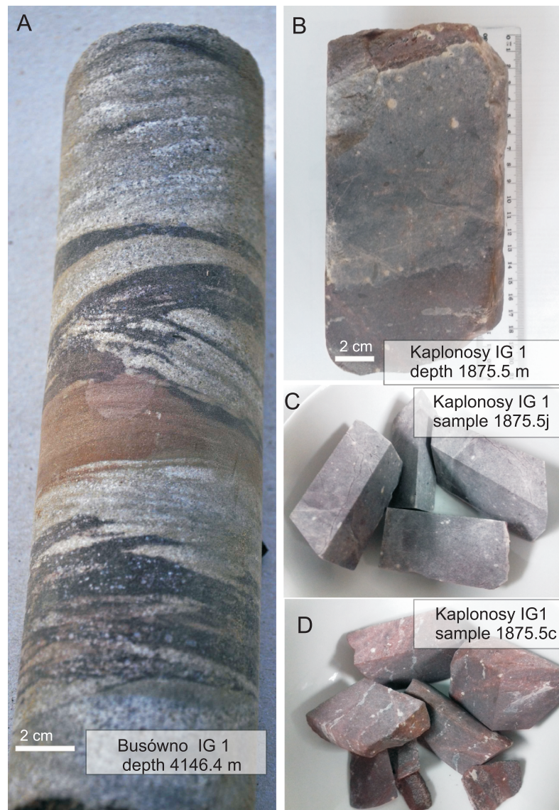
Fig. 3. The drill core samples showing a typical feature of arcose sandstones from the Polesie formation
