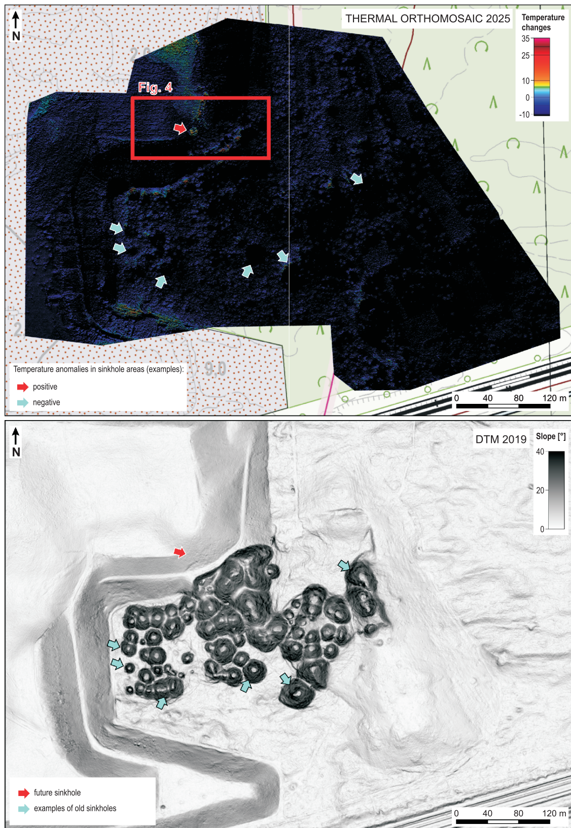
Fig. 3. Thermal orthomosaic and Digital Terrain Model for the test area A
