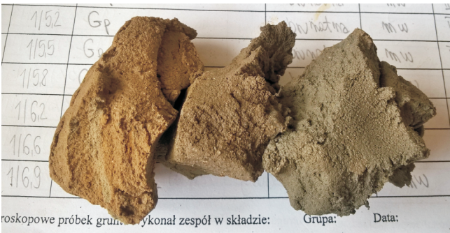
Fig. 7 Till samples during macroscopic examination, from the left: yellow-brown layered North Polish Glaciation tills (ablational), brown North Polish Glaciation tills (basal), Middle Polish Glaciation grey till
