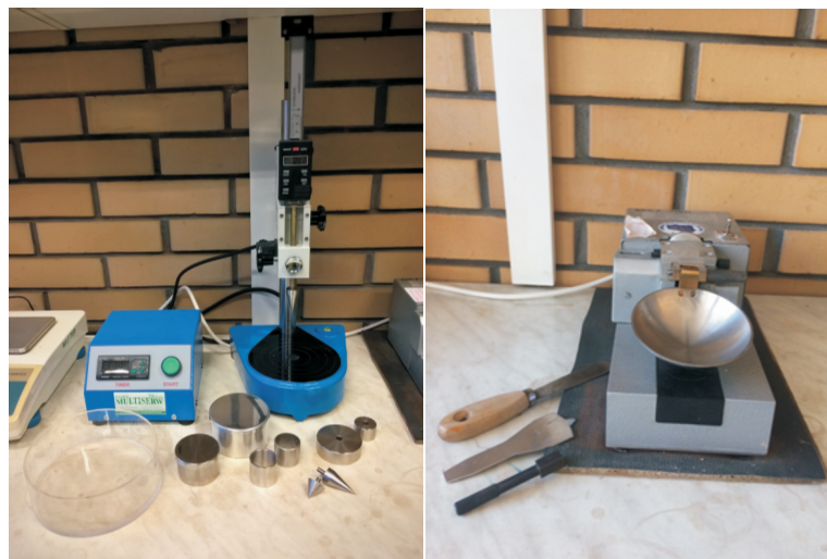
Fig. 10. Tools used to determine the liquid limit value: a mechanically driven Casagrande apparatus (left) and a semi-automatic cone penetrometer (right)
