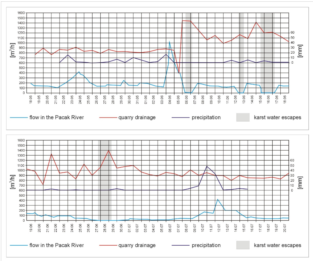
Fig. 13. Episodes revealing response of the gypsum karst aquifer and the Pacak River to increased rainfall recharge (1976)
