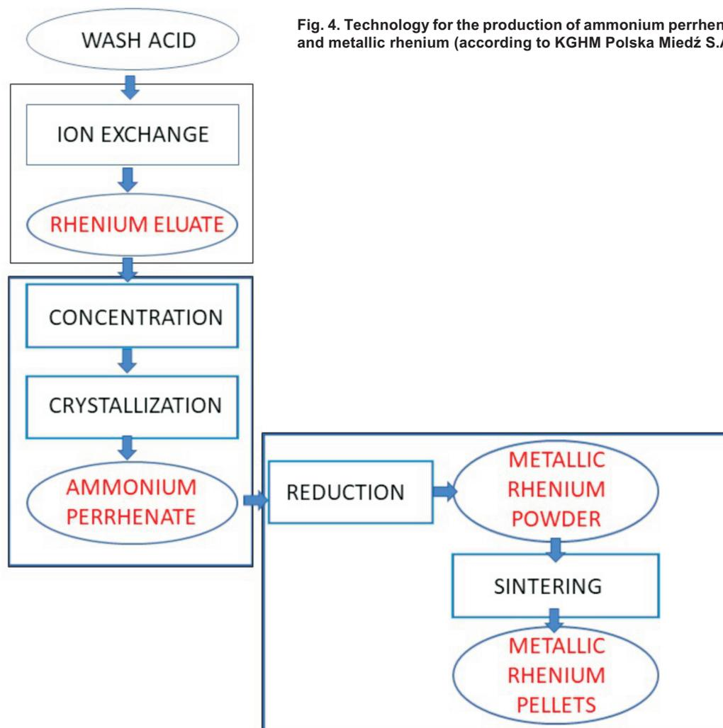
Fig. 4. Technology for the production of ammonium perrhenate and metallic rhenium (according to KGHM Polska Miedź S.A.)
