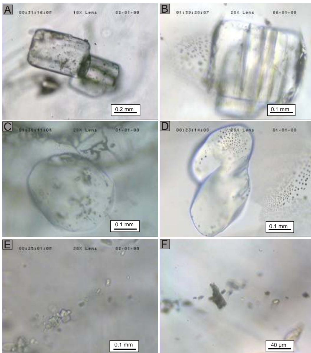
Fig. 3A – large anhydrite crystals of euhedral shape (the first type); B – the same type of anhydrite crystal as in part A with cracks filled with a brown mass; C – the second type of anhydrite crystal, of rounded shape; D – an irregularly shaped anhydrite crystal of the second type; E – very small anhydrite crystals of the third type; F – opaque contaminants in the third anhydrite type as streaks
