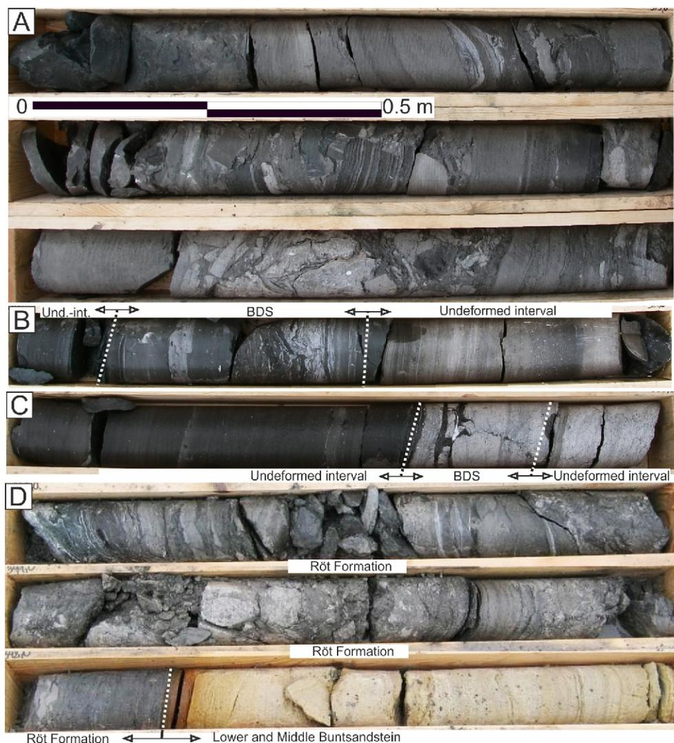
**Fig. 7. Deformation structures in selected core sections**
