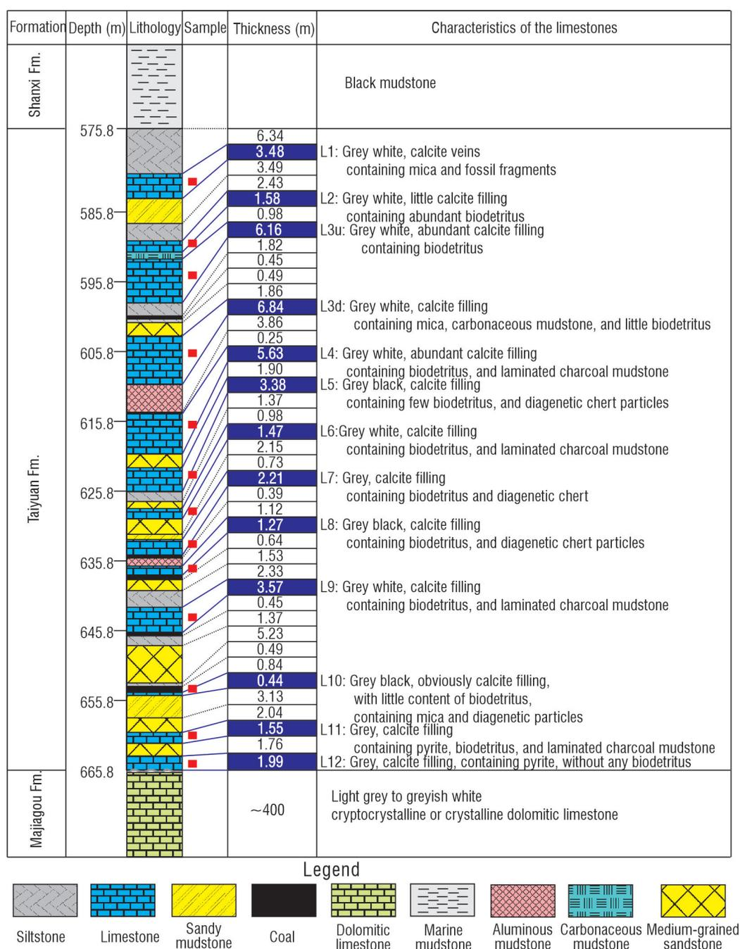
**Fig. 2. Schematic succession and characteristics of the Taiyuan Formation as found in coal-exploration borehole P2 in the Huainan Coalfield (modified after Wu and Zhang, 2019)**
