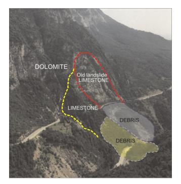
Fig. 4. View of the slope towards the NE with the region of the potential landslide (yellow line)
