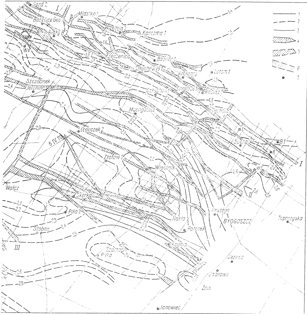
← 1 — isochrone lines of sub-saline boundary — proved; 2 — isochrone lines of sub-saline boundary — tentative; 3 — lines of seismic reflexion profiles; 4 — fault zones of proved course; 5 — fault zones of hypothetical course; 6 — zones of correlation disappearance, related to salt domes; 7 — boreholes
