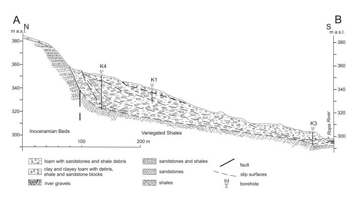
Fig. 5. Geological cross-section of Kawiory landslide
