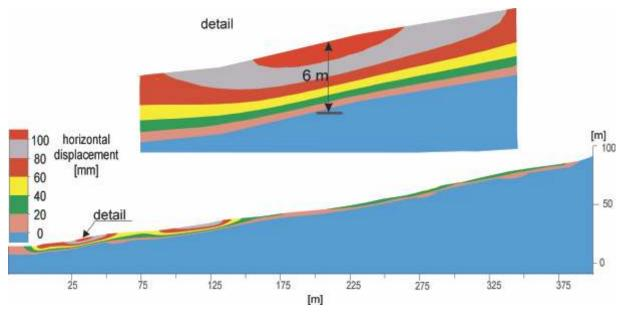
Fig. 13. Field of horizontal displacement after 2 years creep
