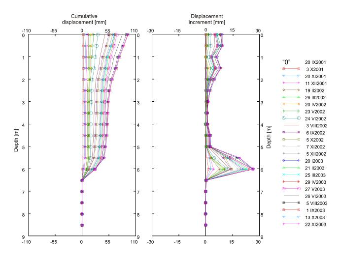
Fig. 8. Cumulative and incremental displacement measured by inclinometer in borehole K3
