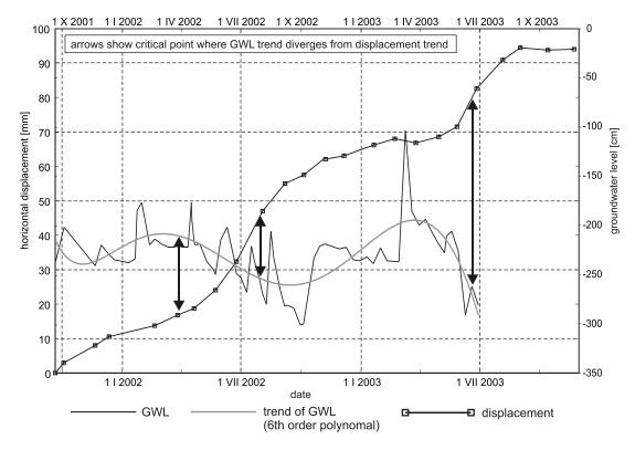
Fig. 10. Groundwater level and horizontal displacement in borehole K3
