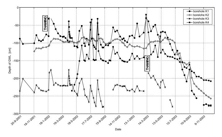
Fig. 7. Groundwater level measured in piezometers
