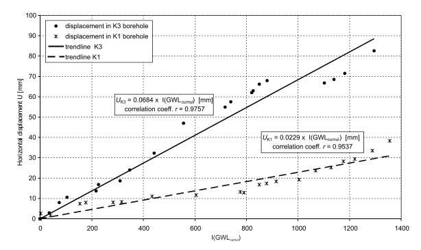
Fig. 11. Cumulative intensity of groundwater fluctuations versus horizontal displacement of K1 and K3 borehole, with regression formula and correlation coefficients
